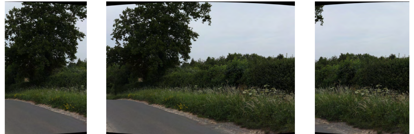
To ensure consistent geometry each image was cylindrically re-projected, as above. This ensures that a full 360 degree panorama can be created to match the 3D model view, as shown below:
